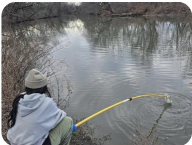
Sampling at a lake edge with an extension pole.
