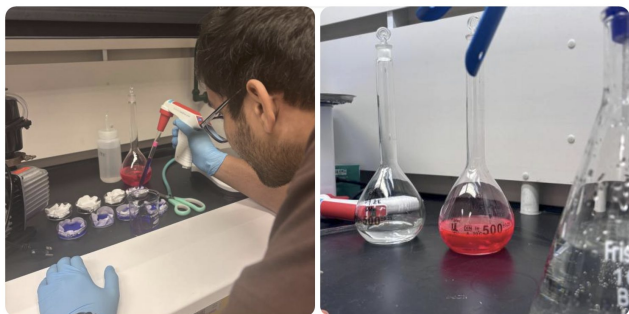
Particle staining (left) and Nile Red dye with Fenton (right).
