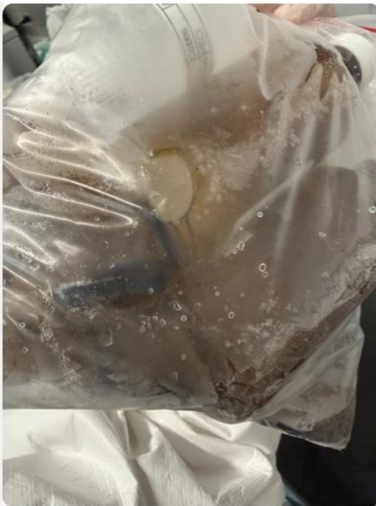
A burst frozen sample, bagged after the jar fractured.
