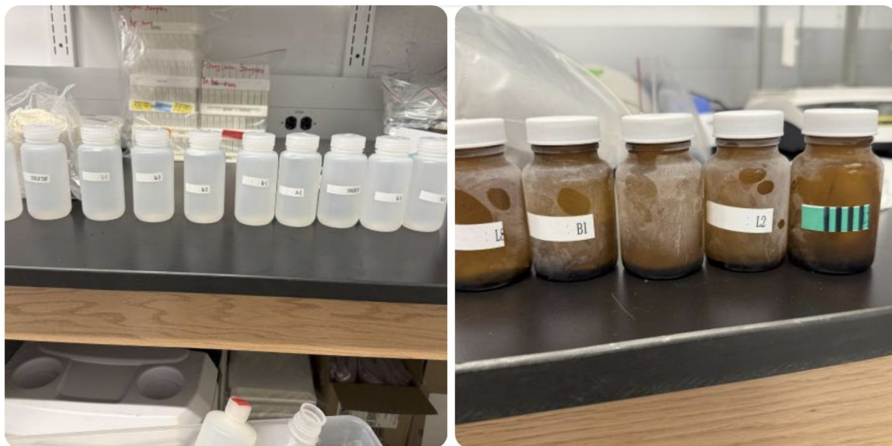
Samples in Nalgene bottles before acidification (left) and frozen samples in amber bottles (right).
